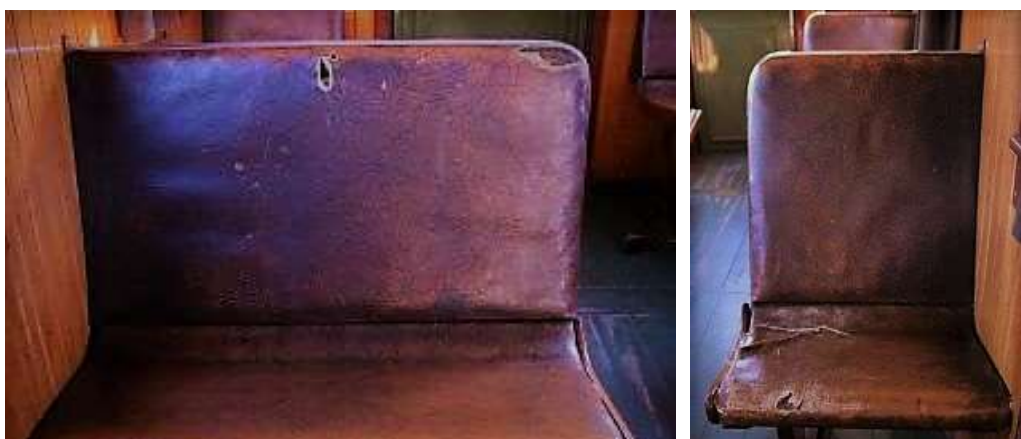
Figure 4-3: Examples of the damage found on the seats. Photographer: Kine E. B. Haugmâne
